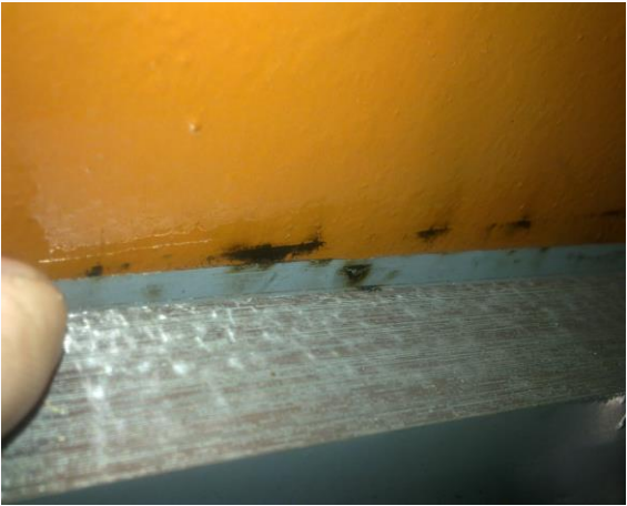
Figure 4: Real Example #2 - Partial Discharges between shunt and tank
