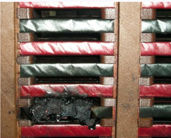
Figure 3: Real Example #1 - Thermal Fault on a 250 MVA autotransformer
