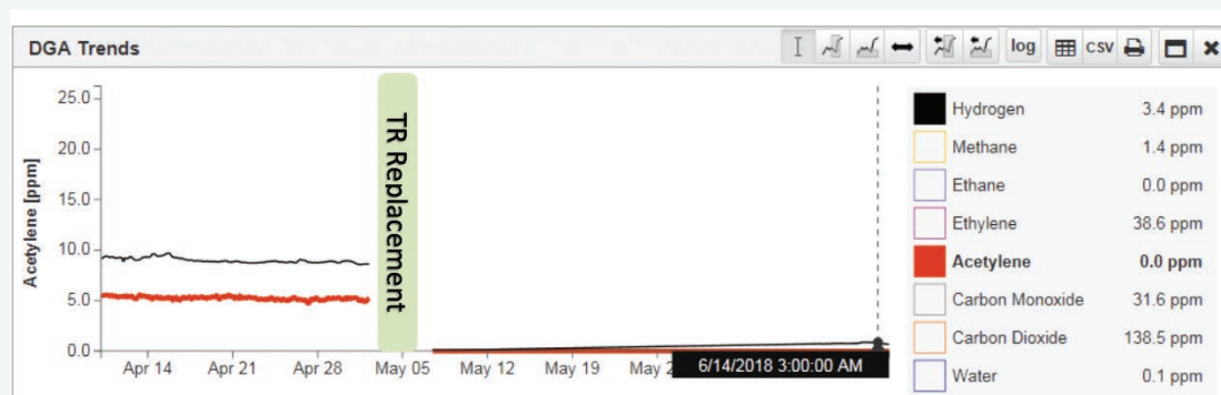
Figure 4: DGA Behavior following the OEM intervention.
