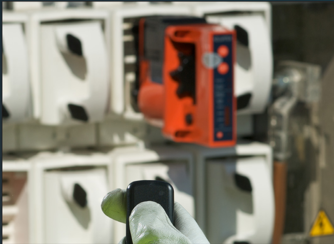
FUSEMATE remote operation via included key fob
