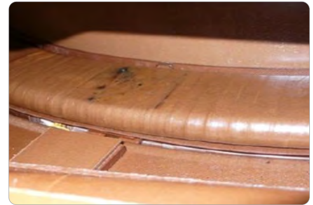
Figure 4 – Carbon tracking appearing on a portion of the transformer winding after oil removed. Presence of tracking indicates that PD activity was present on the winding in this location.
